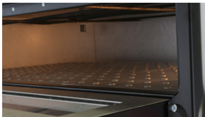
Piano in lamiera bugnata / Buckled plate
